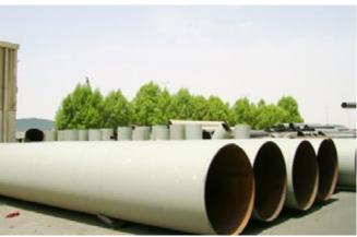
Coating process is a method of protecting blasted surfaces by airless spray application at high pressure utilizing a range of coating systems to suit diverse requirements of the product. The process is applicable to all blasted surfaces of the steel core. The thickness of dry coating of pipe after the coating application of core component is measured based on ASTM D1186 non-destructive measurement of dry film thickness.
