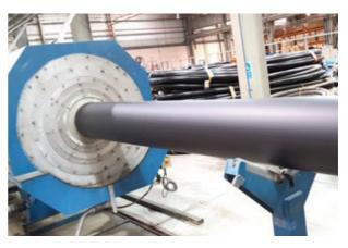
EPPI plastic division manufacture High Density Polyethylene Pipes (EPPI-PE) using the most reliable extrusion machineries. EPPI-PE ranges from (OD) 20mm to 1200mm and the PN from 6 bars to 25 bars.
