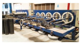
EPPI is equipped with the facility to produce tubular shrinkable HDPE coupling (Rayjoint). The standard size sranges from 90 mm to 1600 mm in diameter. The Rayjoint system has successfully undergone sandbox test as per EN489.
